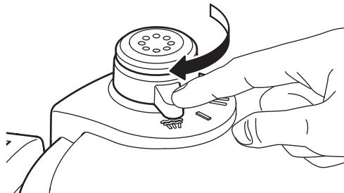
3. Wait until the pressure has equalised and the red safety valve 4 falls back down.
