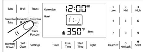
For best results, preheat oven when using convection roast mode.
