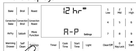
2. Once "12/24" begins to flash in the display, use the numeric touchpad and press 1 (for 12 hr) or 2 (for 24) time scale.
