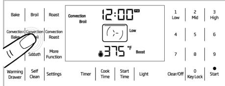
For best results, preheat oven for 5 to 6 minutes when using the convection broil mode. Turn items once while cooking. Broiling time will vary based on size, weight, thickness, starting temperature, and personal preference of doneness.
