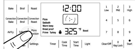
This oven function is available by pressing "More Functions" on the touchpad until the function illuminates on the display.
