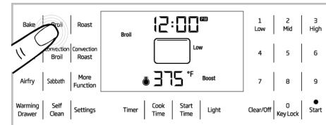
For best results, preheat oven for 5 to 6 minutes when using the broil mode. Turn items once while cooking. Broiling time will vary based on size, weight, thickness, starting temperature, and personal preference of doneness.
