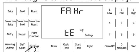
2. Once "F/C" begins to flash in the display, use the numeric keypad to select the desired temperature scale - 1 ( $^{\circ}\text{F}$ ), or 2 ( $^{\circ}\text{C}$ ).
