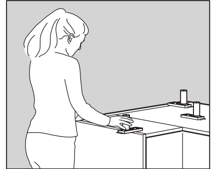
Assemble all base cabinets according to the assembly instructions. Make sure to have the legs attached in the order the cabinets will be installed.
