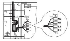
i Tighten the terminal screws securely!
