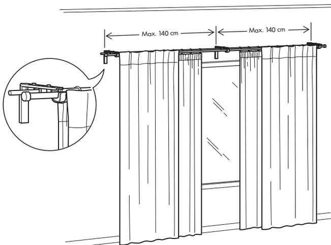
A wide window, for example 280 cm, with a double-layer solution – sheer curtain inside and thick curtain outside.
