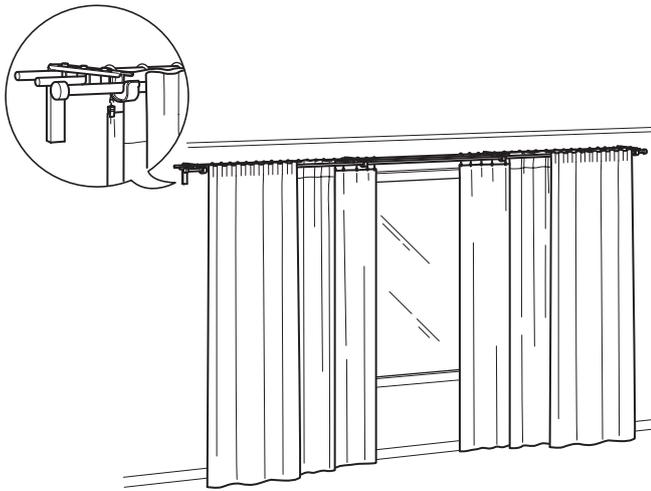
A large window, for example 320 cm, with a triple-layer solution. This configuration allows room for panels, sheer curtains and heavy curtains at the same time.
