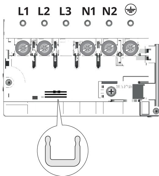
Insert the shunts
