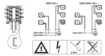
$\bigcirc$  Insert the shunts  $\square$  between the screws as shown.
