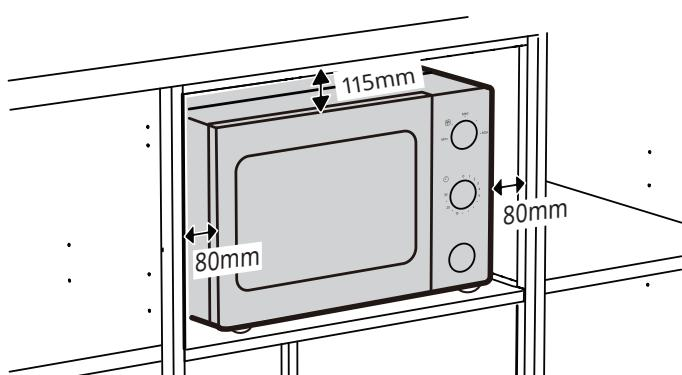
(1) The rear surface of appliance shall be placed against a wall. Leave a minimum clearance of 11.5 cm above the oven, a minimum clearance of 8 cm is required between the oven and any adjacent walls.
