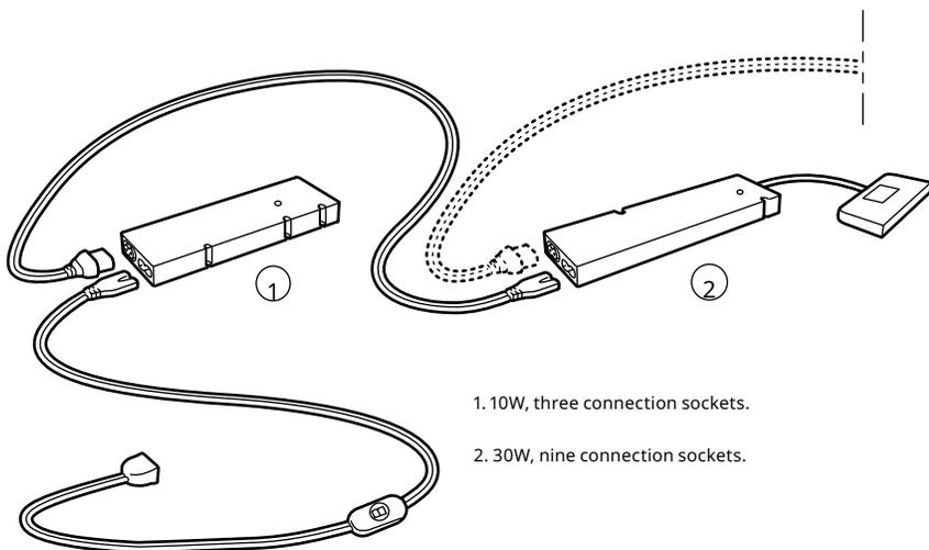
There are two LED drivers. Choose based on how many units you want to connect. You can connect up to three units to the 10W LED driver, as long as the total wattage does not exceed 10W. The 30W LED driver can support up to nine units, max. wattage 30W. You can connect up to ten drivers in one installation cord. Flashing lights indicate that the maximum wattage of the LED driver is exceeded. If you want to use more
