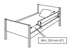
To eliminate the risk of entrapment always fit the guard rail so that it is touching the bed head. The distance between the other end of the guard rail and the foot of the bed must not be less than 230 mm (9").
