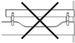
To avoid creating a dangerous gap where children can become trapped, the guard rail must only be used on beds with a straight side rail. The gap between the bottom edge of the guard rail and the top edge of the side rail must not be more than 69 mm (2 3/4").
