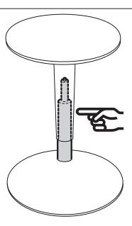
**English**Warning! Only trained personnel may replace or repair seat height adjustment components with energy accumulators.
