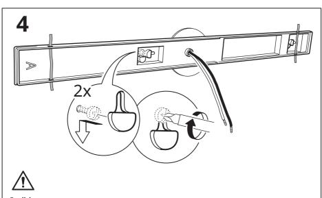
**English**A covering cap or lid must be used if the back of the lamp does not completely cover the wall box.
