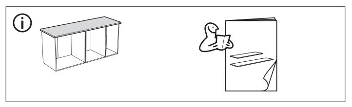
NOTE! Silicone is not included! In order to prevent water from penetrating into the countertop in case of leakage, the cut edges must be sealed with silicone.
