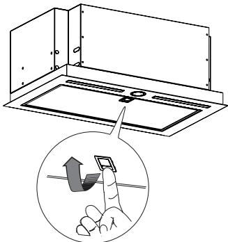
**Replacing the lamps**
