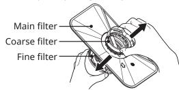
3. Rinse the filter under running water to remove larger food remnants. For more thorough cleaning, use a soft cleaning brush.
