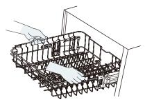
2. To lower the upper basket, lift the adjusting handles on each side to release the basket and lower it to the lower position.
