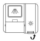
Remove the rinse aid reservoir cap by lifting the handle.
