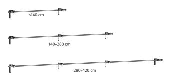
The maximum length between 2 brackets is 140 cm. If your solution is longer, add a bracket for every 140 cm. This means use 3 brackets for curtain rods 140–280 cm; and 4 brackets for rods between 280–420 cm.
