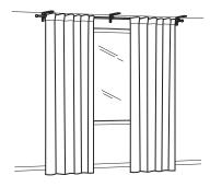
BETYDLIG brackets and curtain rod holders carry max. 10 kg when placed 140 cm apart and the weight of the curtain is evenly distributed over the curtain rod.
