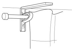
When the brackets are ceiling mounted, you can choose any arm length to adapt the distance between the curtain and window, but you can only mount 1 curtain rod holder.
