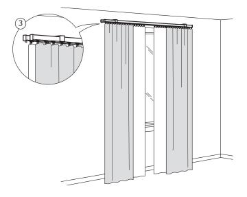
**3.** Two VIDGA single track rails, both 140 cm wide, mounted to the long wall fittings in parallel. By using two layers of curtains, you will have privacy day and night – close the sheer curtains in the day and the outer curtains for the night.
