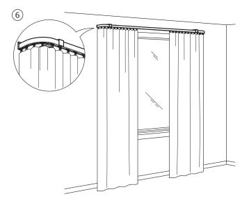
**6.** One VIDGA single track rail 140 cm mounted to the wall. With a corner piece on each side you can pull the curtains all the way to the wall to keep the light completely out.
