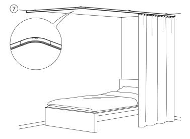
**7.** Three VIDGA single track rails, all 140 cm wide, are connected and mounted to the ceiling. Curtains around the bed create a cosy, private corner.
