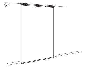
**2.** One VIDGA triple track rail 140 cm mounted to the ceiling. Three VIDGA panel curtain holders are used to attach three panel curtains to the tracks. This combination can be used to cover a window or an open storage solution, or as a room divider.
