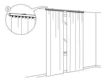
**1.** One VIDGA single track rail 140 cm mounted to the ceiling. The curtains are attached using VIDGA glider and hook.
