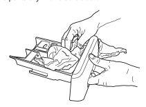
Reinstall the detergent dispenser and push it back into the detergent compartment.
