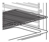
Place the AirFry wire shelf on the third shelf position. Place the baking tray underneath.
