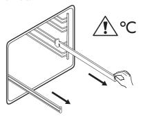
Put the wire shelf on the telescopic runners and carefully push them into the oven. Make sure you push back the telescopic runners fully in the oven before you close the oven door.
