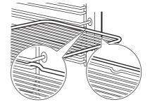
Insert the shelf between the guide bars of the shelf support and make sure that the feet point down. Make sure that the shelf touches the back of the oven interior.
