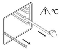
2. Put the wire shelf on the telescopic runners and carefully push them into the oven. Make sure you push back the telescopic runners fully in the oven before you close the oven door.
