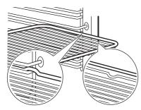
Insert the shelf between the guide bars of the shelf support and make sure that the feet point down. Make sure that the shelf touches the back of the oven interior.
