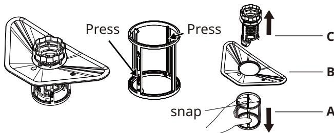
3. Rinse the filters (A), (B) and (C) with water. If necessary, use a soft cleaning brush.
