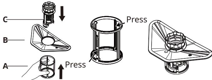
5. Insert the filter assembly into position, and turn it clockwise until it locks. Make sure the arrows on the filter (B) and (C) are aligned, as shown in the figure below.
