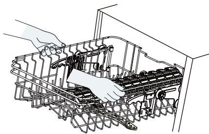
2. To lower the upper basket, lift the adjust handles on each side to realease the basket and lower it to the lower position.
