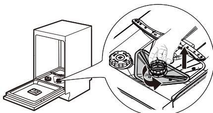
2. First pull the filter (A) out of the filter assembly by compressing the two bars without snap, Then the filter (B) and (C) can be detached.
