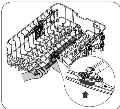
To attach the lower arm spray to the bottom of the appliance, insert the lower arm spray into position.
