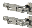
UTRUSTA hinge with built-in damper for kitchen 153°, 2-p. This hinge has an integrated damper, so that the door closes slowly, softly and silently. You can easily deactivate the damper with a side button, for example if you want to use a push opener or if the door closes too slow, and re-activate it if you want. 104.272.62
