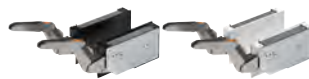
UTRUSTA hinge with damper for horizontal door, 2-p. This hinge has an integrated damper, so that the door closes slowly, softly and silently. You can easily mount the door front in the right position, because the hinges are adjustable in height, depth and width. Snap-on hinges can be mounted onto the door without screws, and you can easily remove the door for cleaning.
