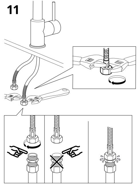
IMPORTANT! Do not tighten too hard: this can damage hoses/pipes and washers.
