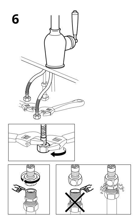
**English**IMPORTANT! Do not tighten too hard: this can damage hoses/pipes and washers.
