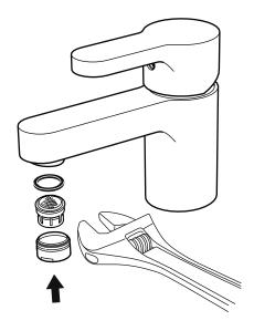
Before use: Unscrew the Aerator/Flow Guide and allow the water to run freely for a few minutes. Then screw the Aerator/Flow Guide back in place. Ensure that it is tight to prevent removal by hand.
