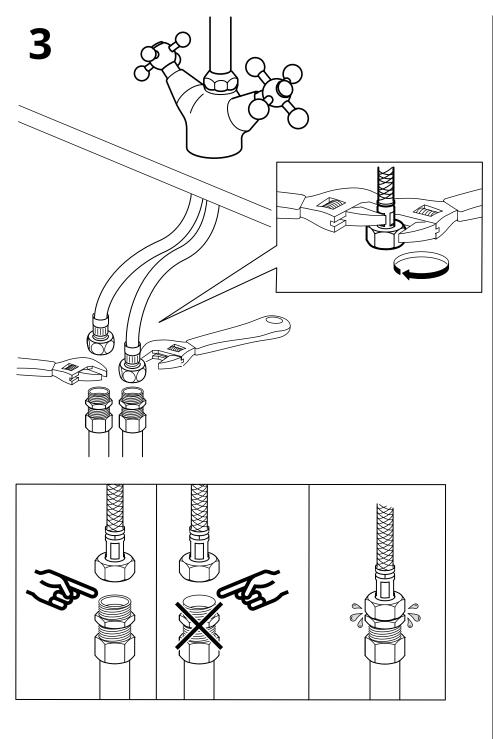
**English**IMPORTANT! Do not tighten too hard: this can damage hoses/pipes and washers.
