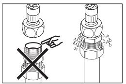
**English**IMPORTANT! Do not tighten too hard: this can damage hoses/pipes and washers.
