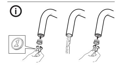
**English**Before use: Unscrew the Aerator/Flow Guide with a coin and allow the water to run freely for a few minutes. Then screw the Aerator/Flow Guide back in place up to the stop DO NOT OVER TIGHTEN.
