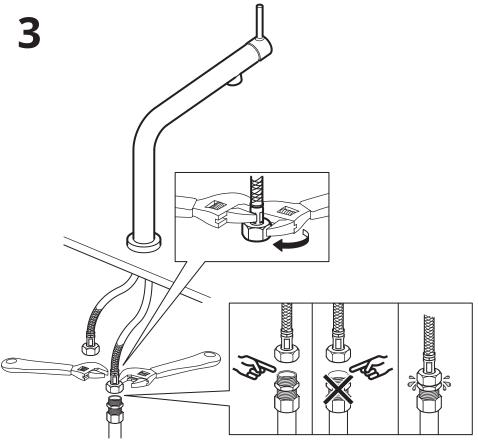
**English**IMPORTANT! Do not tighten too hard: this can damage hoses/pipes and washers.
