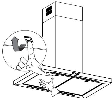
**Replacing the lamps**
