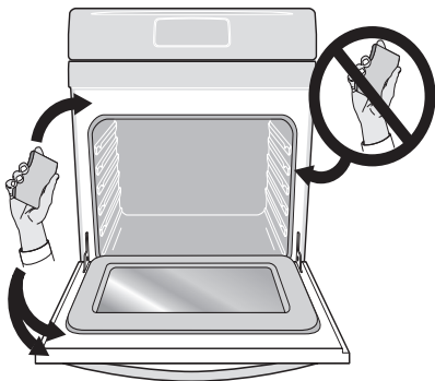
Figure 5: Clean around oven door gasket
