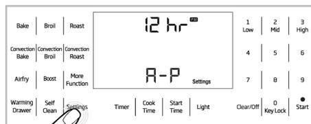
2. "Once "12/24" begins to flash in the display, use the numeric touchpad and press 1 (for 12 hr) or 2 (for 24) time scale.
