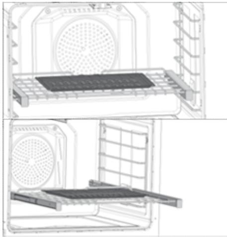
**How to remove the wire shelf with telescopic roller-rack**
