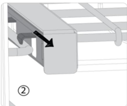
**How to reattach the wire shelf with telescopic roller-rack**
