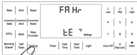
2. Once "F/C" begins to flash in the display, use the numeric keypad to select the desired temperature scale, 1 (°F), or 2 (°C).
