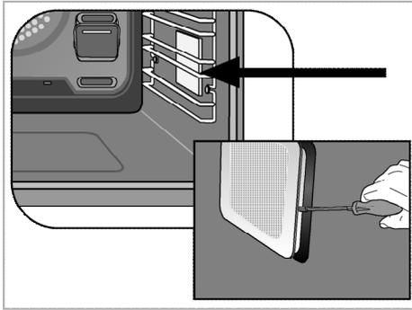
3. Remove the protective glass cover with a screwdriver.
