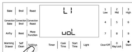
2. "Once "VOL" begins flashing in the display, use the numeric touchpad to choose the desired volume - 1 (low), 2 (med.), or 3 (high).
