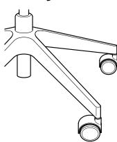
Chairs should stay where you leave them and not roll away on their own. That's why we put safety casters on our chairs. The casters have a built-in pressure-sensitive brake mechanism so that they roll freely and easily when you sit on the chair – and brake when you stand up. Note that even though the casters don't roll when braked, they can still slide on the floor if the chair is pushed.
