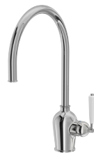
INSJÖN kitchen faucet with sensor H15¾". Swivel spout is preset to 360° but can be changed to 120°. Also available without sensor function or with pull-out spout.
