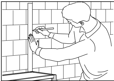
After you have installed the sink cabinet, draw a vertical line from the side of the sink cabinet.
