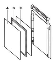
Make sure that you install the middle panel of glass in the seats correctly.
