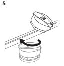
Turn the cap of the salt container clockwise to close the salt container.
