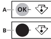
For proper storage of food the refrigerator is equipped with the temperature indicator. The symbol on the side wall of the appliance indicates the coldest area in the refrigerator.
