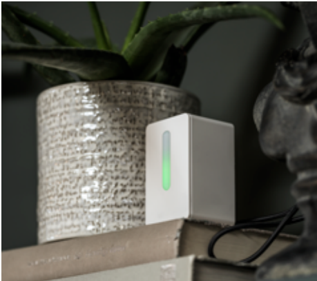
The VINDRIKTNING sensor checks the air quality by detecting particles (PM 2.5 ) in the home.
