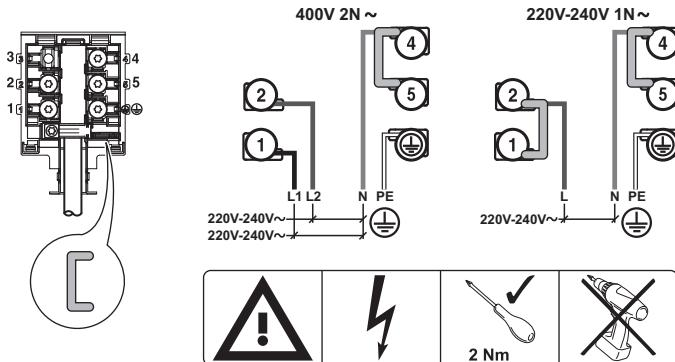
**i** Insert the shunts
