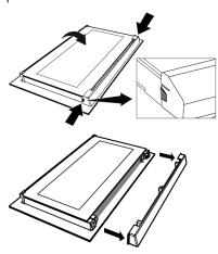
**3.** As shown in the figure, gently lift the innermost glass (1) towards "A" and then, remove it by pulling towards "B".
