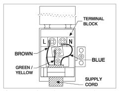
If your supply cord type is 3-conductor type, for 1-phase connection:
