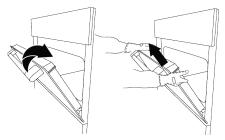
**4.** Pull the removed door upwards to release it from the right and left hinges and remove it.
