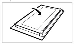
**2.** Pull the plastic component, attached on the upper section of the front door, towards yourself by simultaneously pushing on the pressure points on both sides of the component and remove it.
