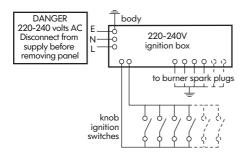
To prevent contact between the cable and the appliance below the hob use the clamps which are on the side of the cabinet.
