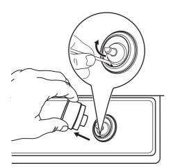
5. To adjust, use a thin bladed screwdriver and turn the adjustment screw until the flame is steady and does not extinguish when the knob is turned from minimum to maximum, and vice versa (see following picture).
