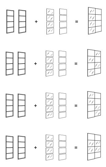
You can also choose your own combination of sliding door metal frames and panels for your sliding doors. The white and black metal frame are only available in the 236 m height. The panels come in a variety of materials and colours. Choose one frame and two packages of panels for each sliding door.
