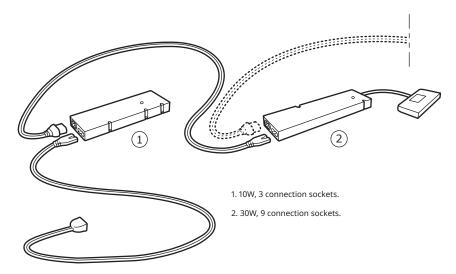
There are two LED drivers. Choose based on how many units you want to connect. You can connect up to 3 units to the 10W LED driver, as long as the total wattage does not exceed 10W. The 30W LED driver can support up to 9 units, max. wattage 30W. You can connect up to 10 drivers in one installation cord. Flashing lights indicate that the maximum wattage of the LED driver is exceeded. If you want to use more than one LED driver,
