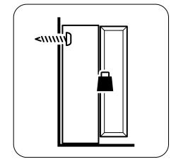
The screw(s) and plug(s) supplied can be used with most solid (A) and hollow (B) walls. For solid wood (C) use the screw(s) without plug(s). If you are uncertain, seek professional advice.
