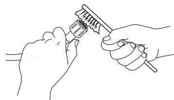
3. Now unscrew the inlet hose on the back of the washing machine by hand. Pull out the mesh filter from the valve on the back of the washing machine with pliers and carefully clean it.
