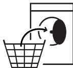
Open the door and load garments. Always refer to instructions on clothing labels and the max loads indicated in the programme section. Empty pockets. Make sure garments do not get caught between the door and/or the door filter.
