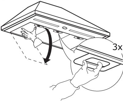
**Replacing the lamps**
