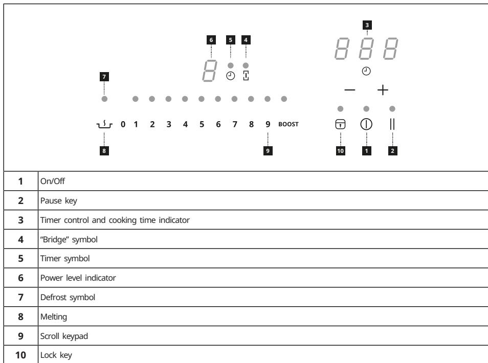
The cooking areas can be activated by pressing the corresponding swipe keyboard. The digit lights up to confirm the operation.
