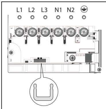
Place shunts between the terminals as shown
