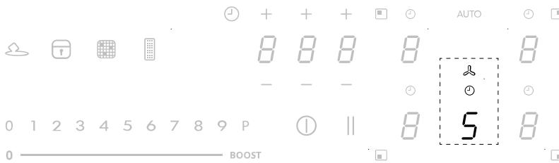
The controls for the cooking zones, extractor and timer can be activated by pressing on the reference Digit.
