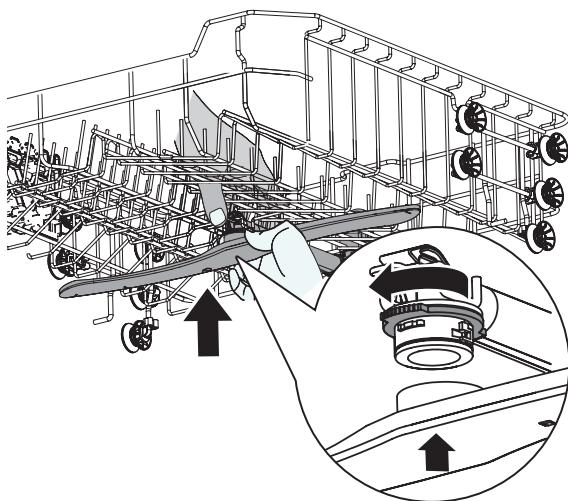
To attach the lower arm spray to the bottom of the appliance, insert the lower arm spray into position.
